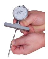
Zeroing the indicator using an extension rod and a setting master.
